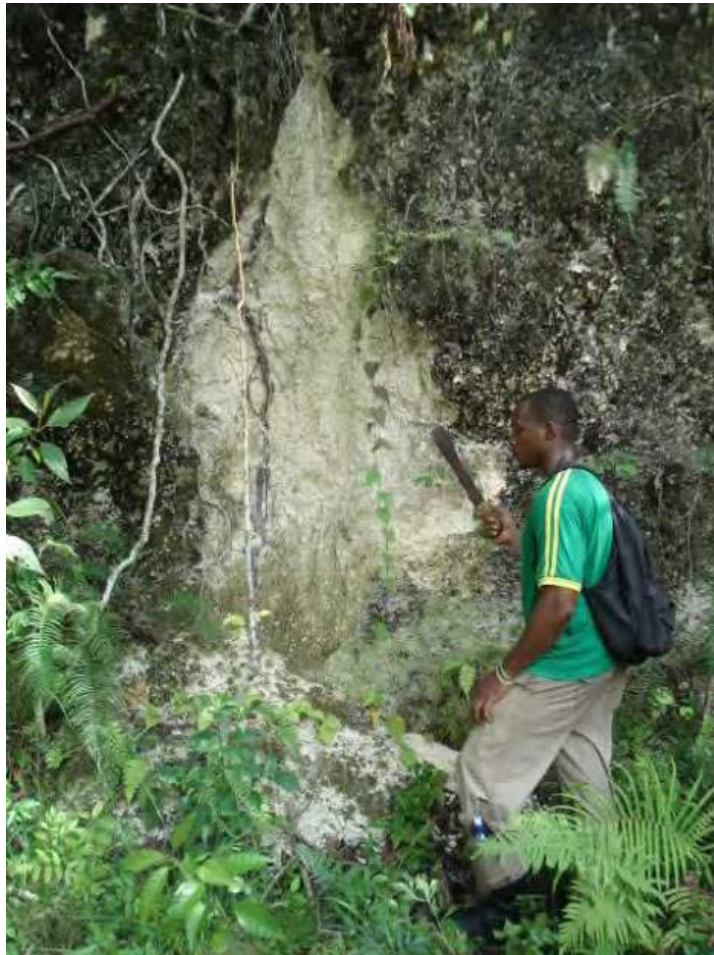
Plate 4.19 - Soft (can be penetrated with cutlass in photo) brecciated material prone to land slips in fault zone (Undifferentiated Troy/Claremont and Somerset formations)
