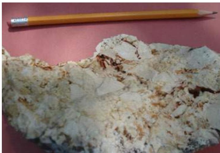
Plate 4.3 - Hand specimen example of the brecciated limestone identified within the Bog Walk Fault zone
